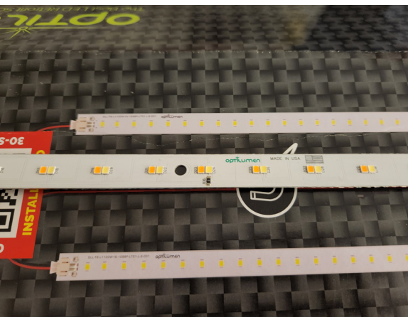
DEC installed magnetic LED retrofit strips at a number of their facilities. These provide a low-cost way to decrease energy use for lighting. Credit: DEC
