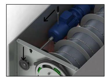
4- With the service brake unlocked, turn the emergency wheel clockwise to turn the brake disk. When you do this, the platform will also rise.
