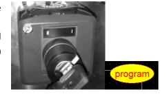
Descend the platform to the first pin position and then press the *Stopover* Key to validate. At that time, *pin1-origin* will be green and the height from the origin will be 0 m. The platform will never stop in this position.
