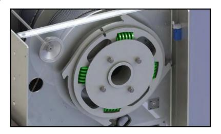
The brake disk is attached to the cable winding drum, from which the platform is suspended.
