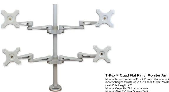
Monitor forward reach is 4" to 21" from pillar center line, monitor height adjusts up to 15"; Steel, Silver Powder Coat Pole Height: 27"
