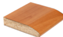
LC-9 2" x 1-1/4" Comfort Eased front edge with 3mm x 1- 1/4" Flat rigid P12 Black Ebony PVC on remaining 3 edges. 1/8" radius corners & edges.
