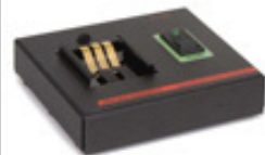
Battery Charger Platform 200-0584-00 For first generation LIDAR and ATR. Charges Ni-Cad & NiMH battery handles. Accepts 015-0194-00 Switching power supply or 019-7058-00 Euro AC Power supply. Full and trickle charge modes for 200-0480-00 battery.
